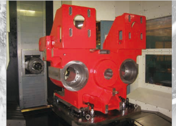
Name : Bearing Housing Material : Casting
