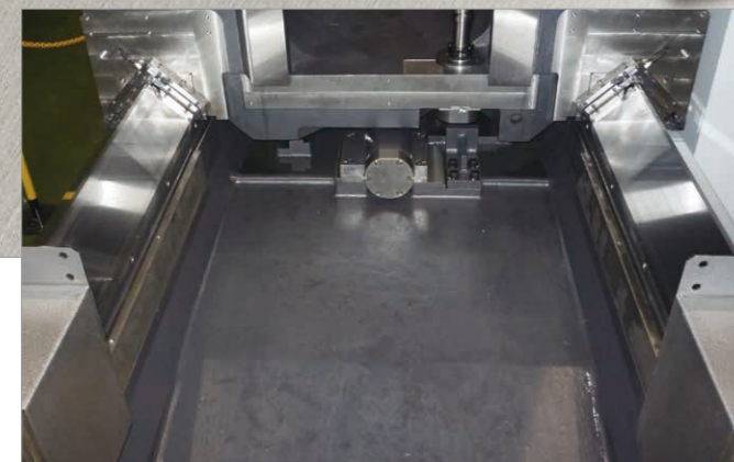
Z axis : V - V shape slide way
